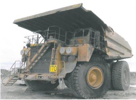
One of two identical rock trucks that recently burned. The fire suppression systems on the trucks failed.
